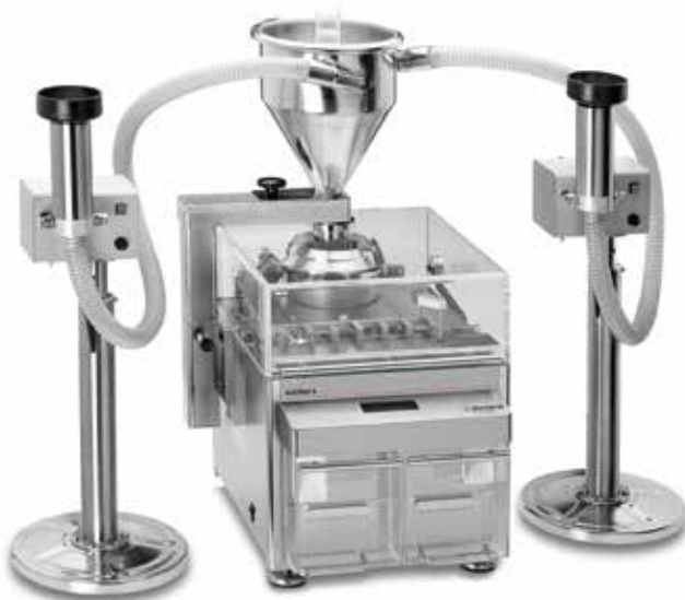
→ Air transport system for a double-sided tablet press: the brake cyclone gently slows down tablet samples arriving at the AutoTest 4
